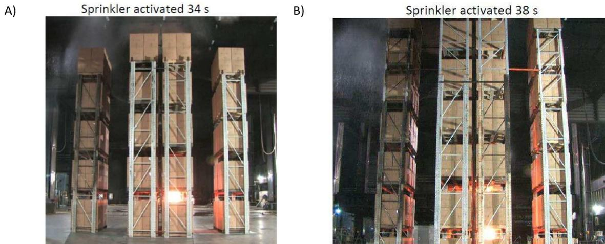
Figure 1: Fire spread at sprinkler activation for previous SMART sprinkler tests<sup>3</sup>; a) fire is below 3<sup>rd</sup> tier for 5-tier configuration; b) fire is below 4<sup>th</sup> tier for 7-tier configuration.
