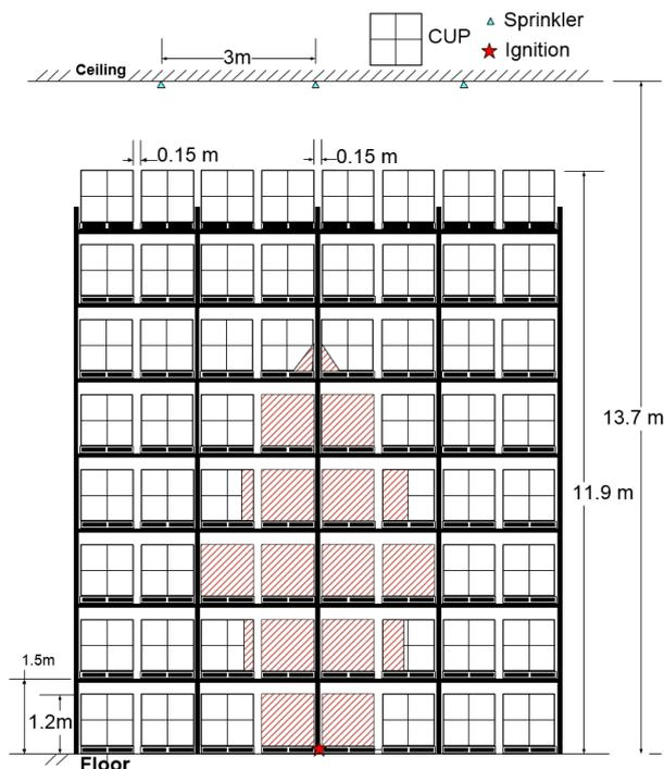
Figure 9: Fire damage of main array represented by red hatch marks (viewed from east). Wooden pallets between each red area were also burned. No fire damage to target arrays was present during testing.
