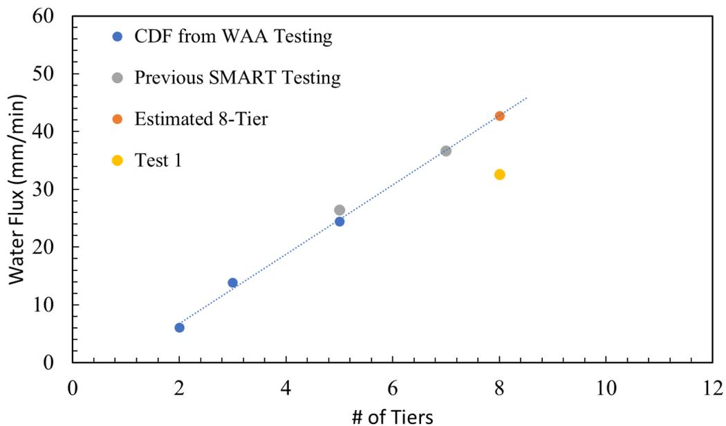
Figure 2: Water density values determined from WAA testing and the previous SMART testing for various tier heights.
