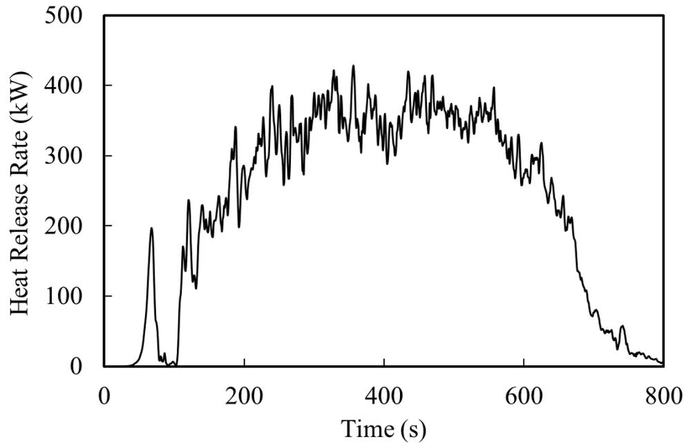
Figure 7: Estimated convective HRR of fire with activation occurring at 62 seconds.
