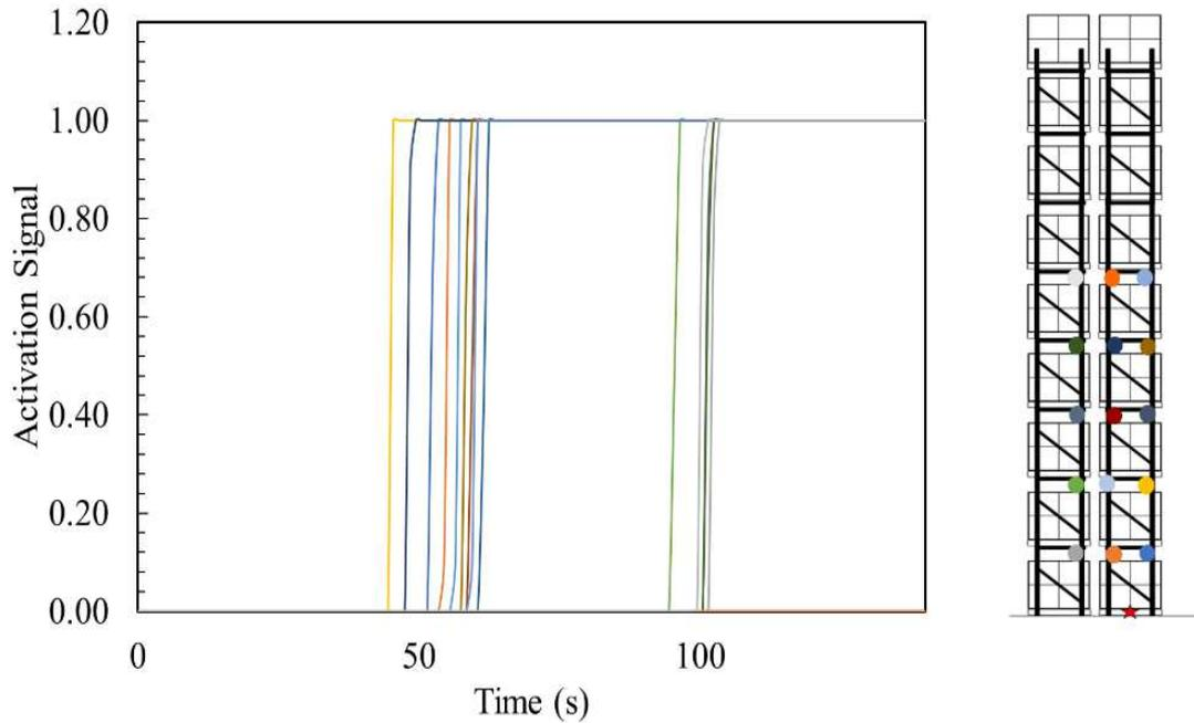
Figure 5: Linear heat detector activation signals from multiple locations and tiers during a traditional sprinkler test. Each color represents a different linear heat detector installed within the array as shown in the side view of the array.
