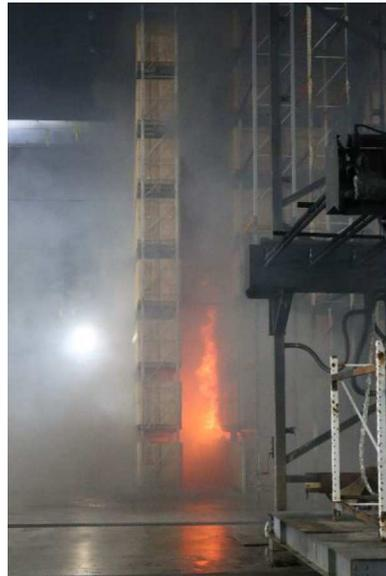
Figure 6: Fire development for 8 tiers of storage with 32.6 mm/min.
