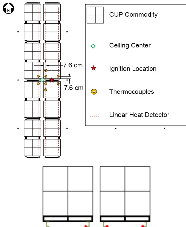
Figure 4: In-rack detection instrumentation showing both thermocouple placement and LHDs, (LHDs placed above first 5 tiers of CUP).
