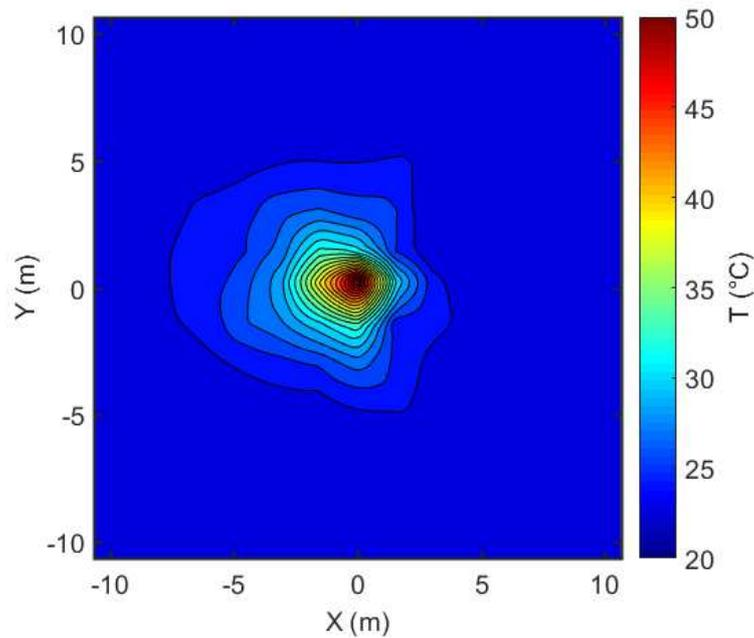
Figure 8: Temperature profile of virtual thermocouples placed 0.3m from the ceiling at sprinkler activation.
