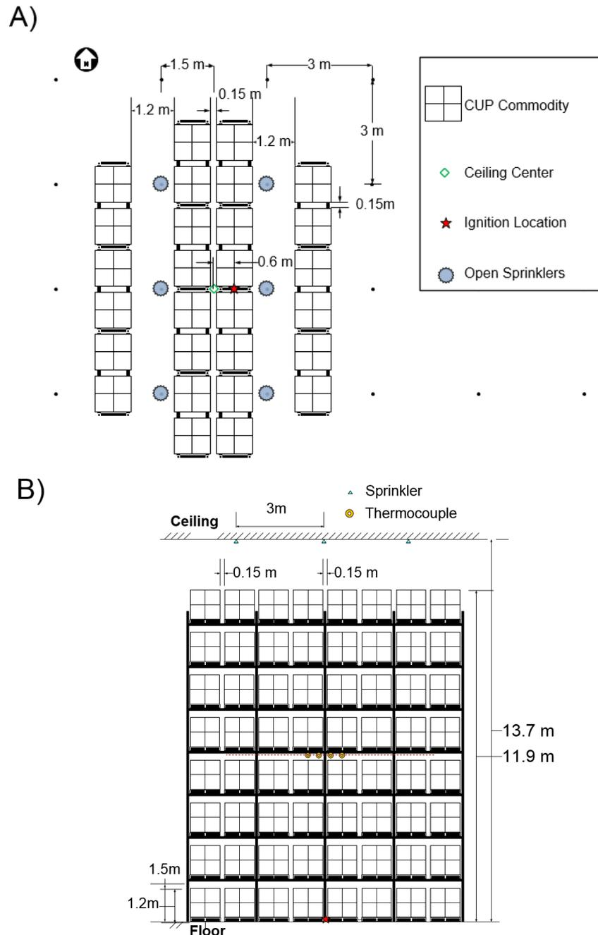
Figure 3: a) Plan view of proposed test setup, utilizing a “between 2” configuration. b) Elevation view of main array used for Test 1: 8 tiers of CUP storage under a 13.7m ceiling.
